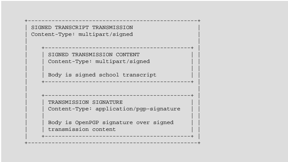
Figure 9: MIME Structure of Signed Transcript Transmission
