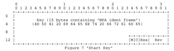
Key: This field contains the "key" used to authenticate that the sender is an MPA sender. Senders must set this field to the fixed value "MPA ident frame" or (in byte order) 4D 50 41 20 69 64 65 6E 74 20 66 72 61 6D 65 (in hexadecimal). Receivers MUST check this field for the same value, and close the connection if any other value is detected.
