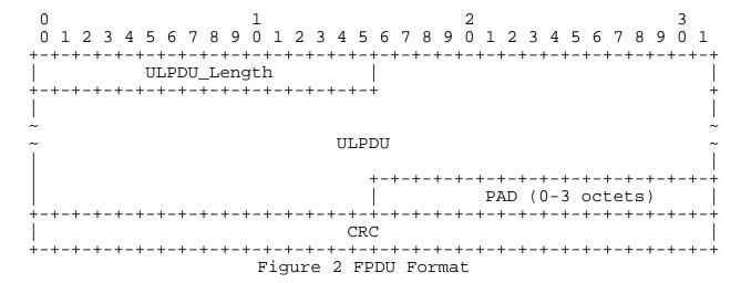
ULPDU\_Length: 16 bits (unsigned integer). This is the number of octets of the contained ULPDU. It does not include the length of the FPDU header itself, the pad, the CRC, or of any markers that fall within the ULPDU. The 16-bit ULPDU Length field is large enough to support the largest IP datagrams for IPv4 or IPv6.
