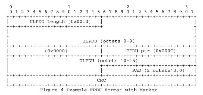
MPA Receivers MUST preserve ULPDU boundaries when passing data to DDP. MPA Receivers MUST pass the ULPDU data and the ULPDU Length to DDP and not the markers, headers, and CRC.
