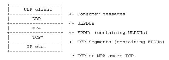
Figure 1 ULP MPA TCP Layering
