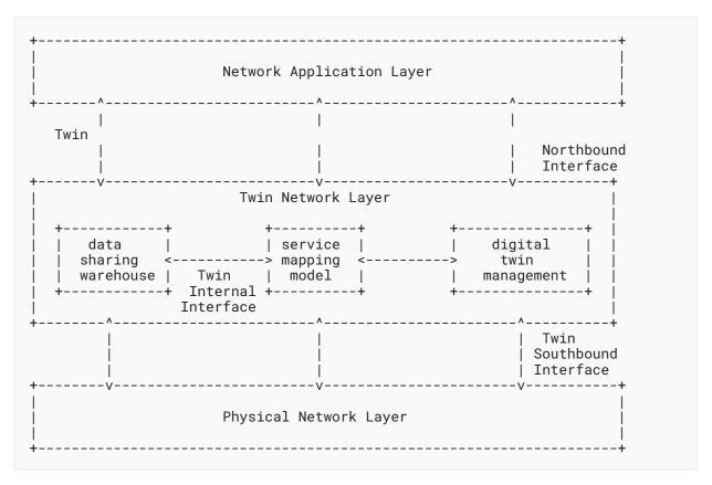
Figure 1: Schematic Representation of DTN Interface
