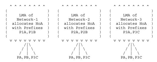
Figure 6. Example of Anycast of HoA Prefixes. The LMA in each network broadcasts the superset of prefixes PA, PB, P3C. Here PA is the aggregate of P1A, P2A, and P3A; PB is the aggregate of P1B and P2B
