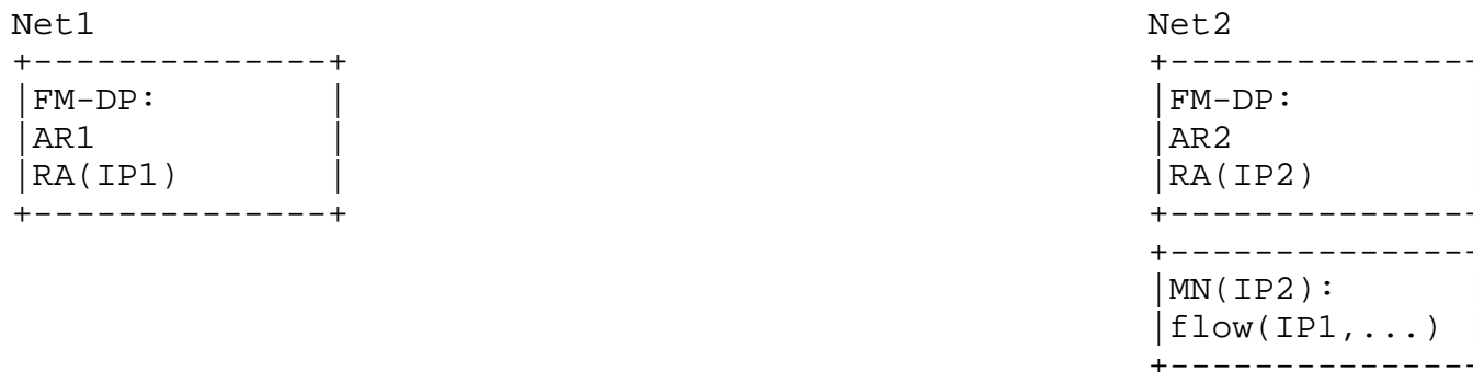
Figure 4. IP address anchored not in network of attachment. MN attached to AR2 in Net2 has a flow(IP1,...) using IP1, which belongs to Net1.
