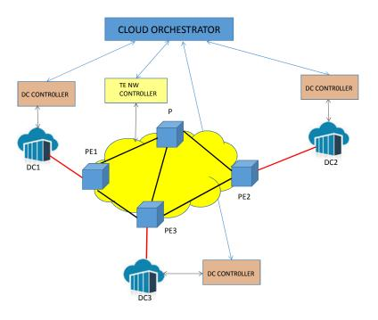
Figure 5 - Data Center Interconnection Use Case
