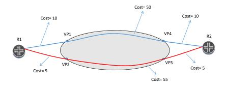
Figure 3 - IP+Optical Path Computation Example
