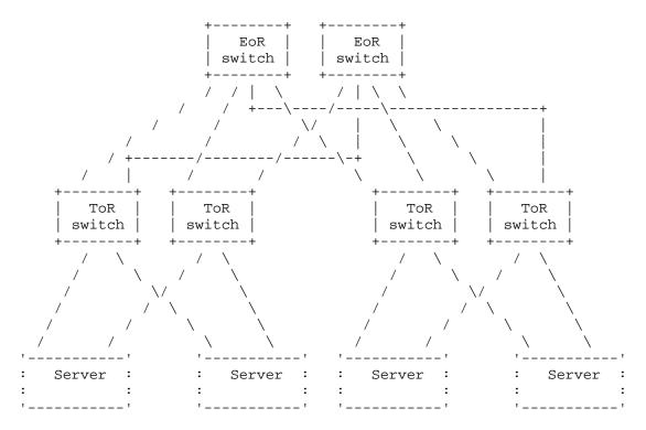
Figure 1: Typical Data Center Mesh Network
