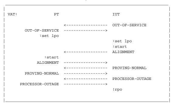
Figure 3.1.11-2. Set RPO when "Aligned Not Ready"
