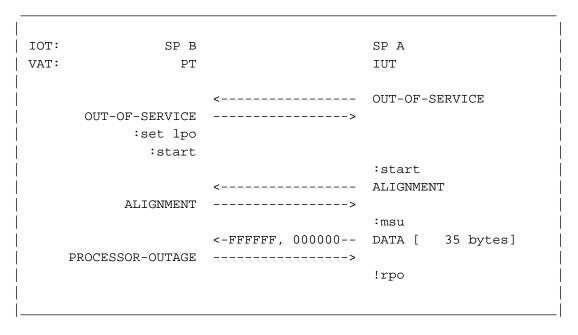
Figure 3.1.9-4. Normal alignment with PO set (Data)
