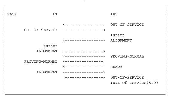
Figure 3.1.33-1. "Alignment" instead of "In Service"
