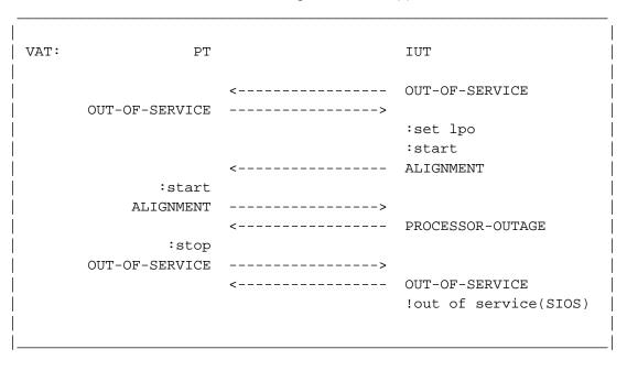
Figure 3.1.12-3. "Out of Service" when "Aligned not ready"
