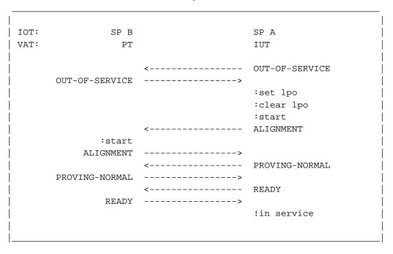
Figure 3.1.10-1. Normal alignment with PO set and cleared
