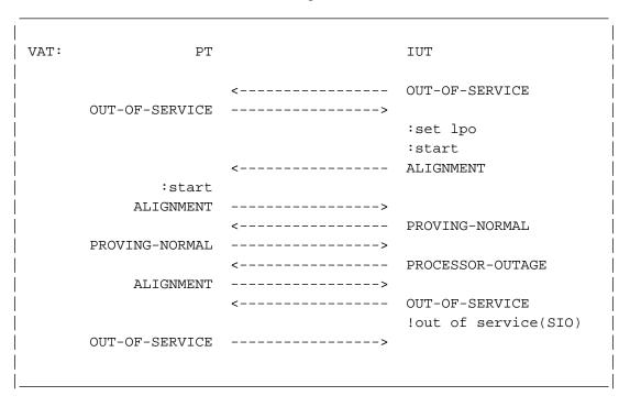
Figure 3.1.13-1. "Alignment" when "Aligned not ready"
