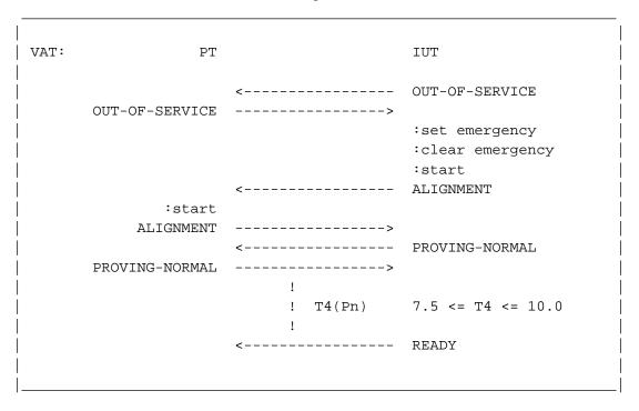
Figure 3.1.18-1. Toggle emergency before "start alignment"
