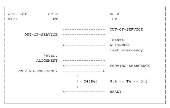
Figure 3.1.19-1. Set emergency in "not aligned" state
