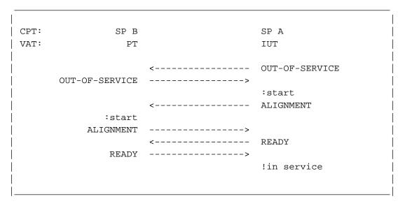
Figure 3.1.5-3. Normal alignment procedure (without proving)
