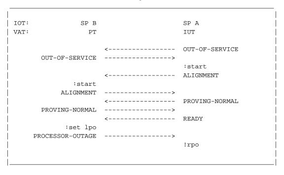
Figure 3.1.35-1. "Processor Outage" instead of "In Service"
