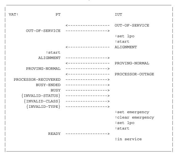
Figure 3.2.6-1. Unexpected events while "aligned not ready"
