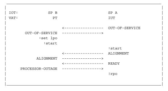
Figure 3.1.8-4. Normal alignment with PO set
