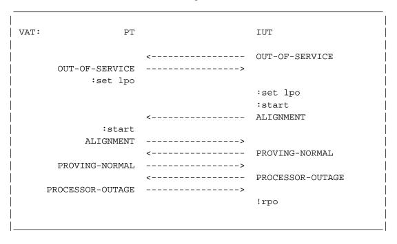
Figure 3.1.11-1. Set RPO when "Aligned Not Ready"
