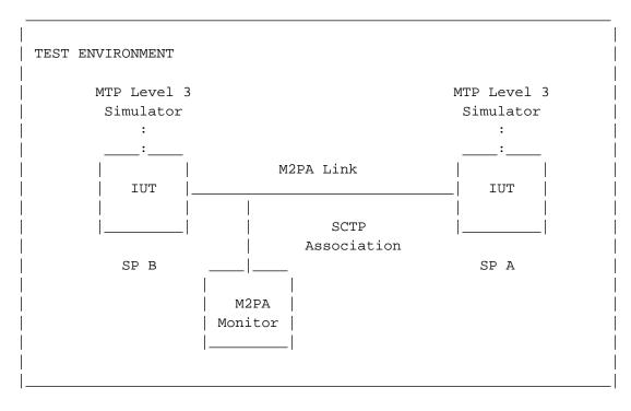
Figure 2.1.2-1. Compatibility Test Configuration
