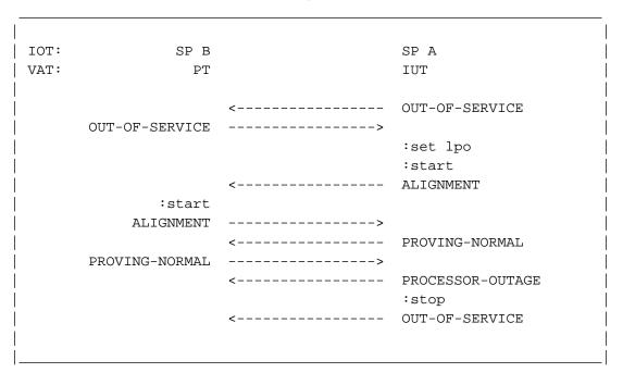
Figure 3.1.27-1. Deactivate during aligned not ready
