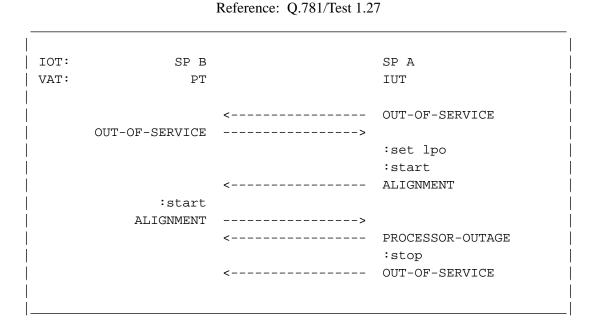
Figure 3.1.27-2. Deactivate during aligned not ready
