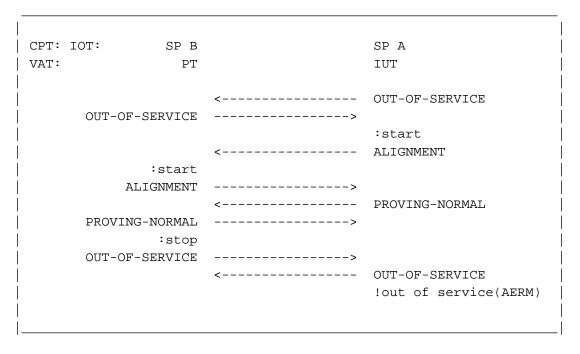
Figure 3.1.32-1. Deactivation during the proving period
