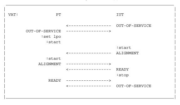
Figure 3.1.12-4. "Out of Service" when "Aligned not ready"
