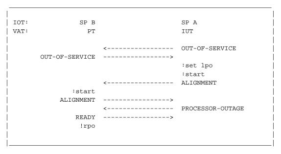
Figure 3.1.8-3. Normal alignment with PO set
