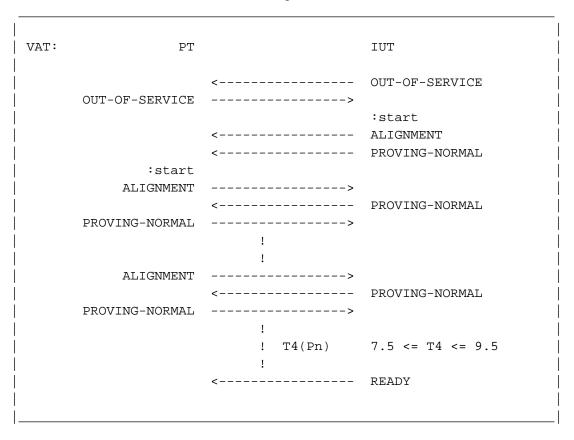
Figure 3.1.7-1. "Alignment" during normal proving
