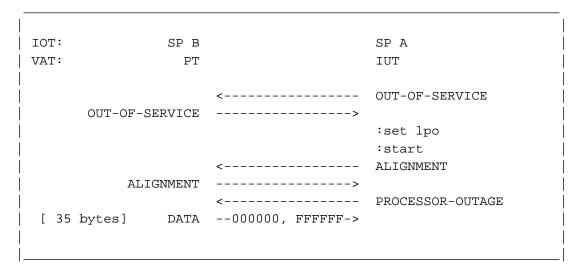
Figure 3.1.9-3. Normal alignment with PO set (Data)
