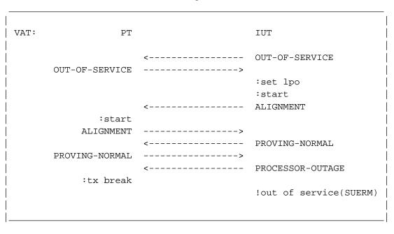
Figure 3.3.3-1. Link aligned not ready (Abort)
