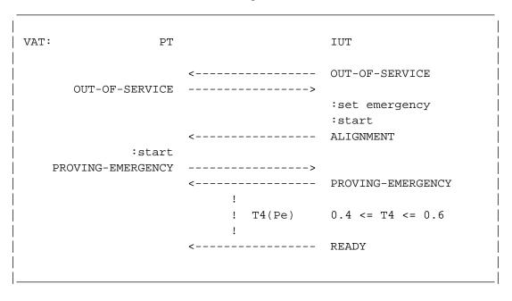
Figure 3.1.24-1. No "Alignment" during emergency alignment
