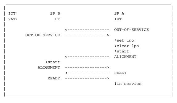
Figure 3.1.10-2. Normal alignment with PO set and cleared
