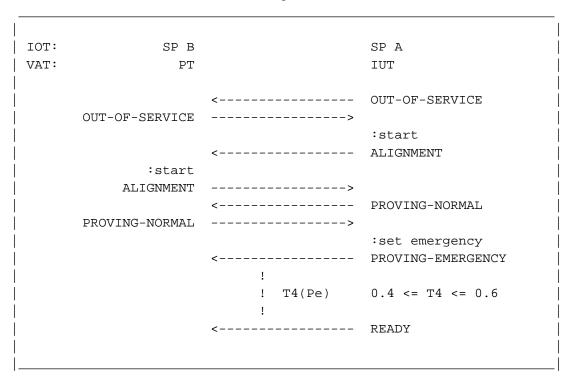
Figure 3.1.20-1. Set emergency when "aligned"
