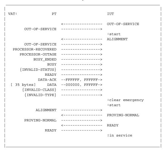
Figure 3.2.2-1. Unexpected events while "not aligned"
