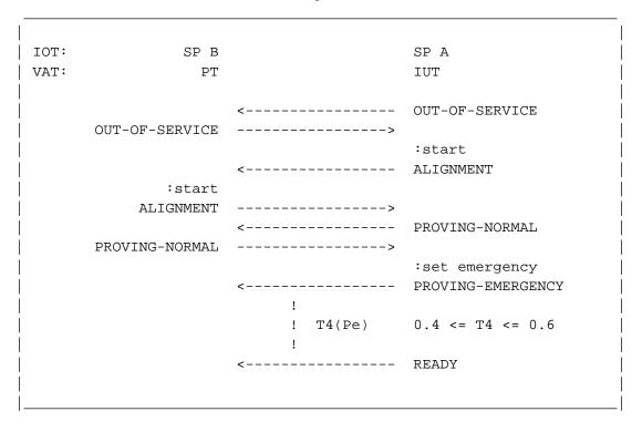
Figure 3.1.23-1. Set emergency during normal proving
