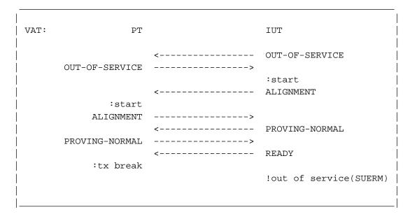
Figure 3.3.1-1. Link aligned ready (Abort)
