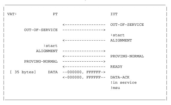
Figure 3.1.6-1. Normal alignment procedure (Data) with proving
