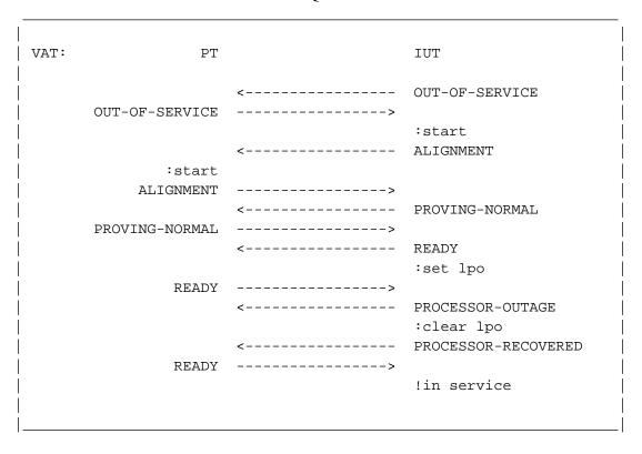
Figure 3.1.15-1. Set and clear LPO when "Aligned ready"
