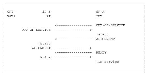
Figure 3.1.5-4. Normal alignment procedure (without proving)
