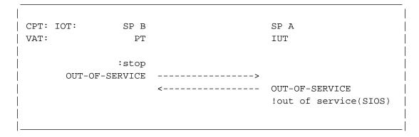
Figure 3.1.29-1. "Out of service" during link in service
