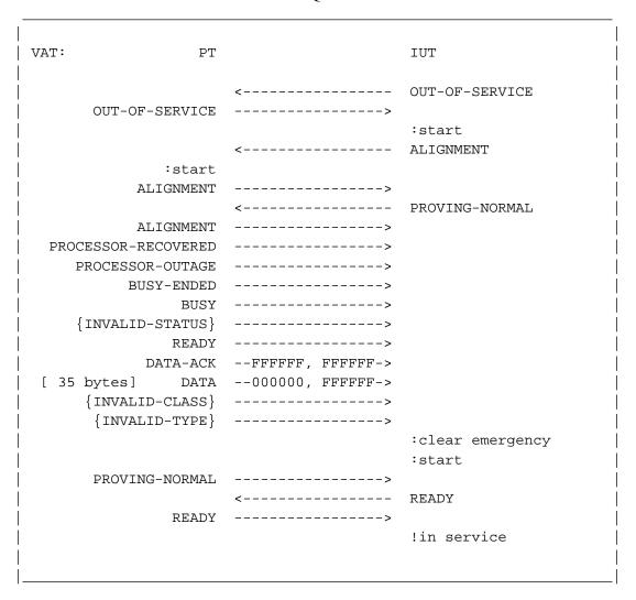
Figure 3.2.3-1. Unexpected events while "aligned"
