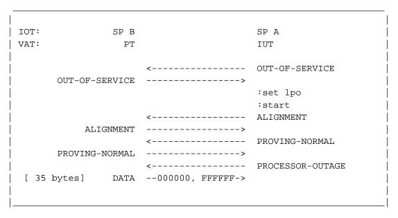
Figure 3.1.9-1. Normal alignment with PO set (Data)
