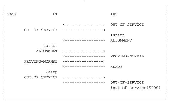
Figure 3.1.34-1. "Out of Service" instead of "In Service"
