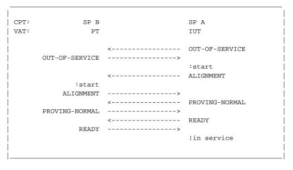
Figure 3.1.5-2. Normal alignment procedure
