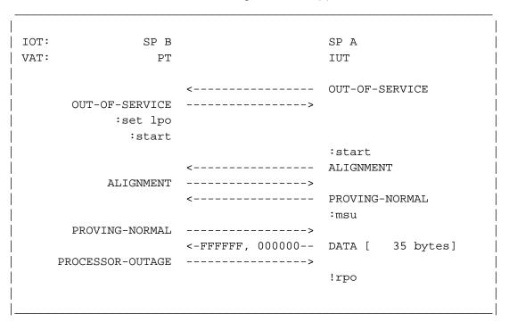
Figure 3.1.9-2. Normal alignment with PO set (Data)
