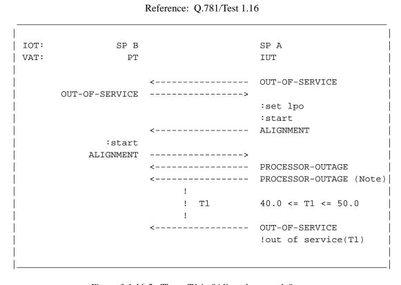
Figure 3.1.16-2. Timer T1 in "Aligned not ready" state
