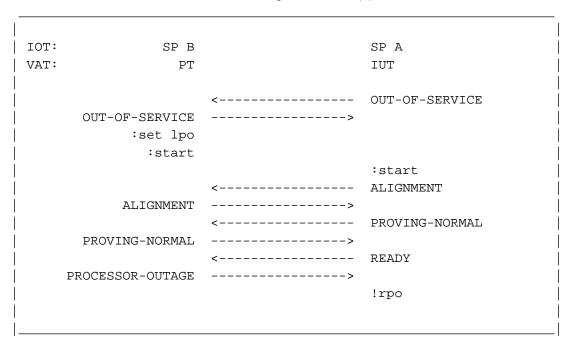
Figure 3.1.8-2. Normal alignment with PO set
