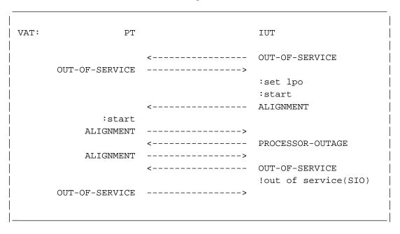
Figure 3.1.13-2. "Alignment" when "Aligned not ready"
