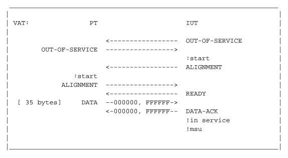
Figure 3.1.6-2. Normal alignment procedure (Data) without proving
