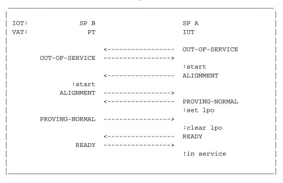
Figure 3.1.14-1. Set and clear LPO when "Initial Alignment"
