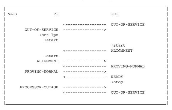
Figure 3.1.12-2. "Out of Service" when "Aligned not ready"
