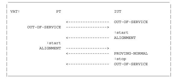
Figure 3.1.26-1. Deactivate during aligned state
