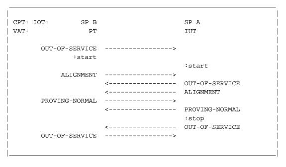
Figure 3.1.32-2. Deactivation during the proving period
