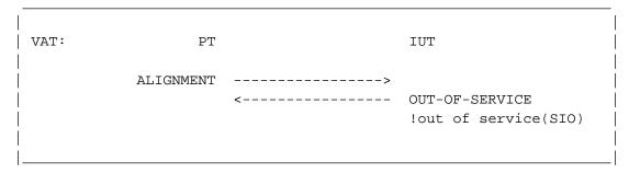
Figure 3.1.28-1. "Alignment" during link in service
