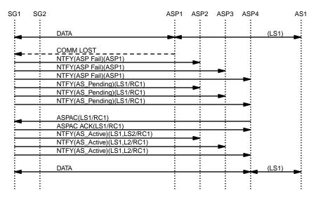
Figure 6. M3UA Example – Failure of ASP1
