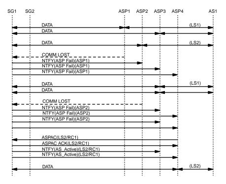
Figure 9. SUA Example - Failure of ASP1 and ASP2
