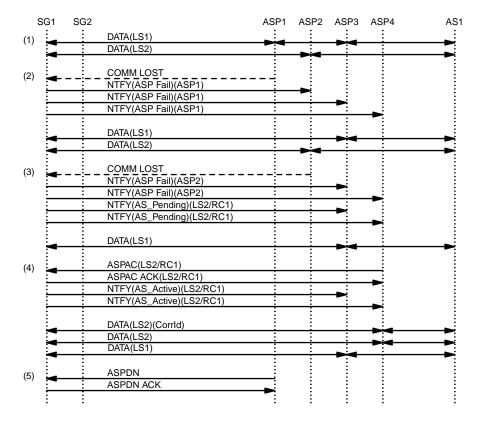
Figure 12. TUA Example – Failure of ASP1
