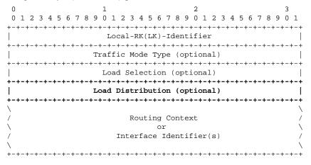
When an ASP wishes to register within a Load Group associated with an Application Server, it includes the *Load Selection* parameter and *Load Distribution* in the *Routing (Link) Key* for that Application Server in the **REG REQ** message.
