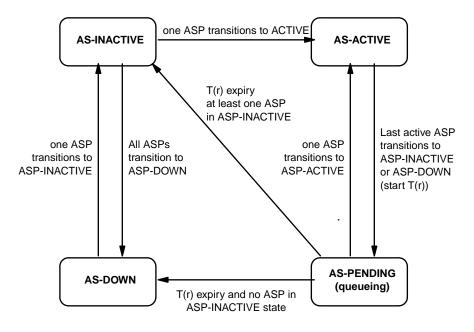
Figure 6. AS State Transition Diagram
