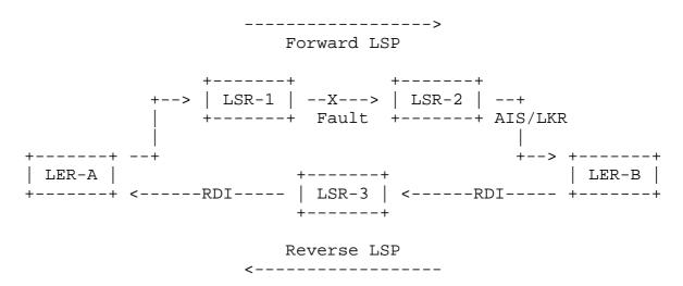
Figure 2: RDI Operation in Associated Bidirectional LSP
