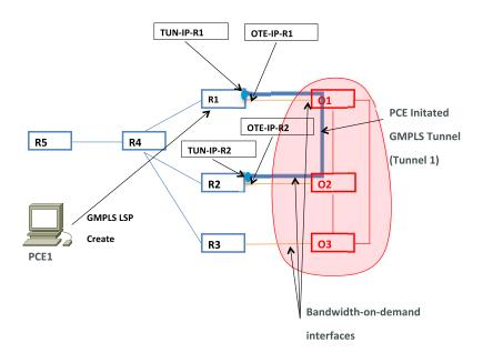
Figure 2. Use case higher-layer signaling trigger
