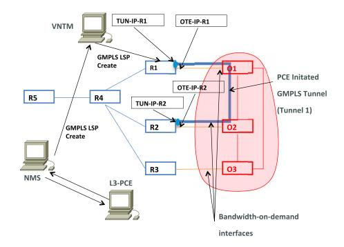
Figure 3. Use case NMS-VNTM cooperation model
