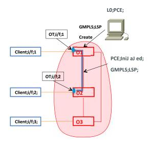
Figure 1. Single-layer provisioning from active stateful PCE.
