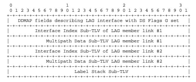
Figure 2: Example of DDMAP in MPLS Echo Reply
